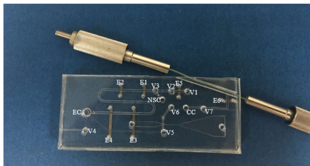
Fig. 11 Image of the lab-on-a-chip system for continuous glucose monitoring. V1-V7 are pneumatic valves. E1-E6 are six pairs of electrodes. EC: Extraction Chamber, NSC: Normal Saline Chamber, CC: Collection Chamber
